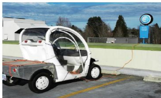
Neighborhood EV at Level 1 EV charging station
